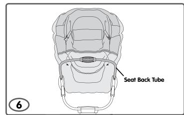
• Fit the upper pocket on the pad around the seat back tube.
